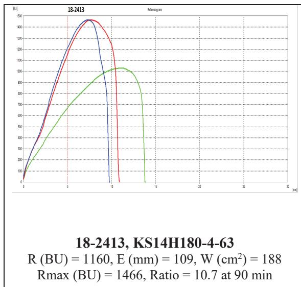
Notes: R (BU) = Resistance; E (mm) = Extensibility; W ( $\text{cm}^2$ ) = Energy; Rmax (BU) = Maximum resistance. Green = 45 min, Red = 90 min, and Blue = 135 min.
