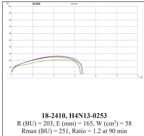
Notes: R (BU) = Resistance; E (mm) = Extensibility; W (cm<sup>2</sup>) = Energy; Rmax (BU) = Maximum resistance. Green = 45 min, Red = 90 min, and Blue = 135 min.
